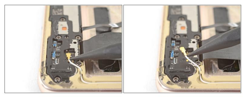
Use the point of a spudger to pry up and disconnect the white antenna cable from the bottom of the phone.
