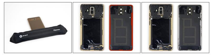
• <u>Heat an iOpener</u> and apply it to the bottom edge of the phone for two minutes. Re-heat the iOpener as needed.
