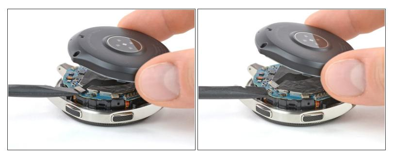
• Use a spudger to disconnect the sensor flex cable from the motherboard.
