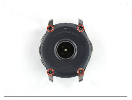
Remove the four Tri-point #00 screws (4.2 mm length) on the backside of the watch.
