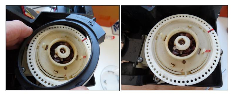
• The grinder is situated on the top right rearside of the device. The adjuster and the outer ring can just be taken off, but this is only necessary if the grinder has to be completely replaced. Be careful and do not use excessive force.
