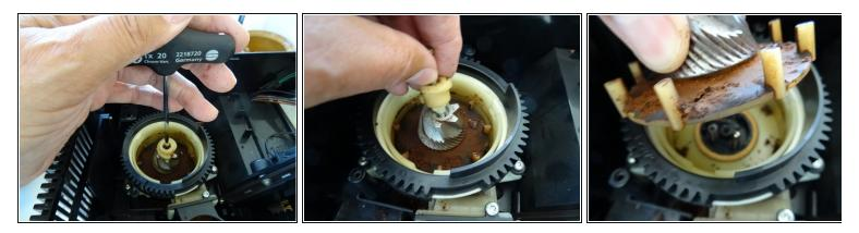
In the next step be very careful not to loose these three springs, balls and cartridges.
