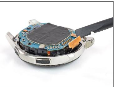
Use a spudger to disconnect the display flex cable from the motherboard.
