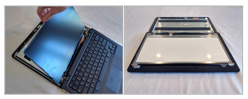
• Carefully separate the LCD panel from the plastic cover. and lower the screen onto the keys.
