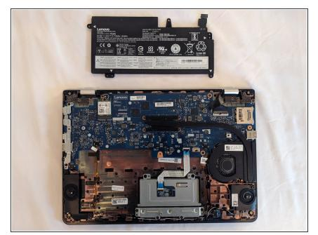
• Lift the battery out of the upper case.
