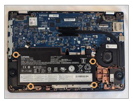
• Remove the four screws securing the battery to the upper case.
