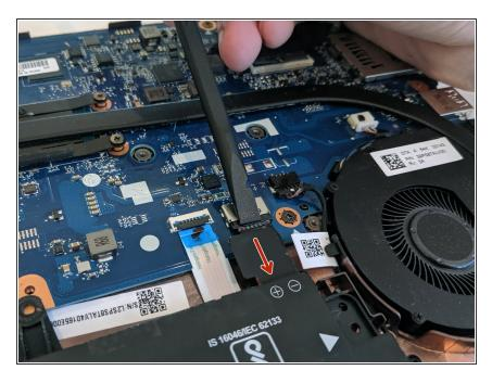
Use a spudger or other plastic tool to push the battery connector in the direction of the arrow, removing it from its socket.
