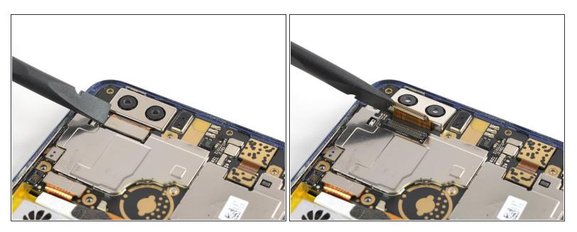
• Use a spudger to pry up and disconnect the rear camera flex cable from its motherboard socket.
