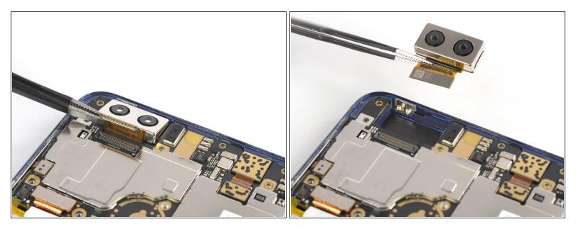
• Use a pair of tweezers to carefully lift the rear camera out of its recess and remove it.
