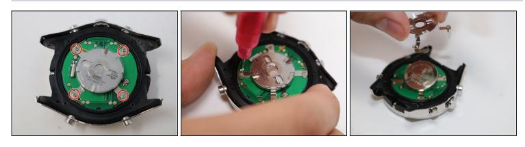
• Remove the four 1.1 mm screws located on the metallic holder using the Phillips #00 screwdriver.
