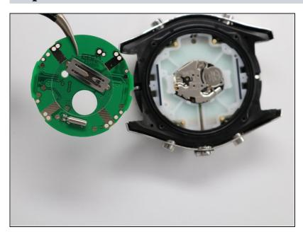
Remove the green circular chip using a pair of <u>tweezers</u>.
