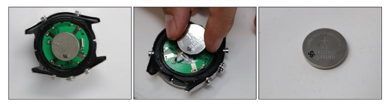
• Remove the large circular Analog battery.
