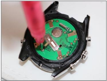
• Using the Phillips #00 screwdriver, remove the two 1 mm screws holding the circuit board to the device.
