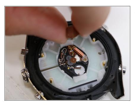
• Remove the digital battery from the socket.
