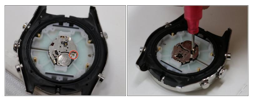
Using the Phillips #00 screwdriver, remove the 1.1 mm screw that is holding the digital battery holder in place.
