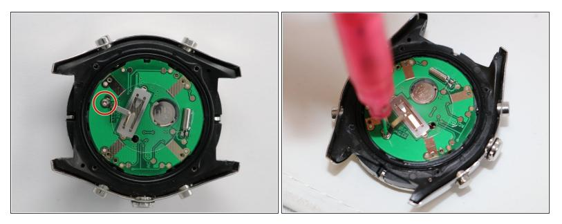
Using the Phillips #00 screwdriver, remove the two 1 mm screws holding the circuit board to the device.
