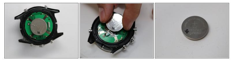
• Remove the large circular Analog battery.
