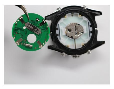
• Remove the green circular chip using a pair of tweezers.
