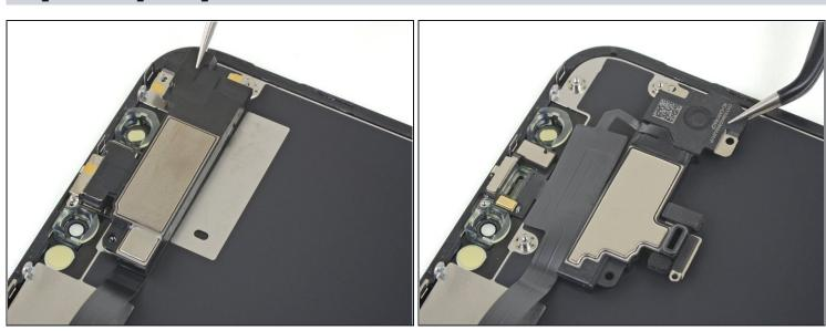
• Using <u>tweezers</u>, gently flip the speaker assembly over—down and away from the top edge of the display.
