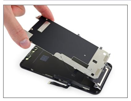
• Remove the LCD shield.
