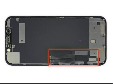
• Apply a little heat from an iOpener (or hair dryer / heat gun) to the back of the display, in order to soften the adhesive securing the display cables to the LCD shield.
