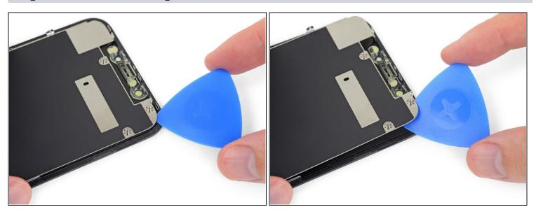
• Insert an opening pick under the top edge of the LCD shield, and twist to separate it from the display.
