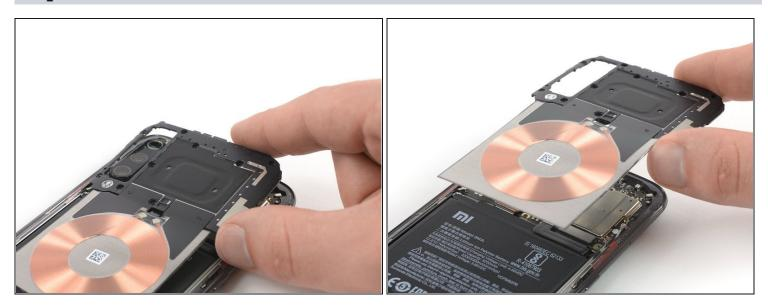
• Carefully remove the motherboard cover including the charging coil / NFC antenna.
