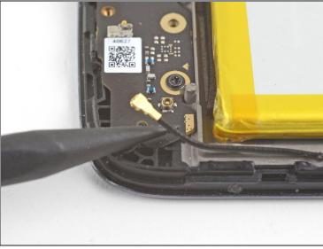
• Use the point of a spudger to pry up and disconnect the antenna cable from its daughterboard socket.
