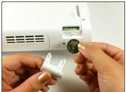
• Pull out the battery holder and battery.
