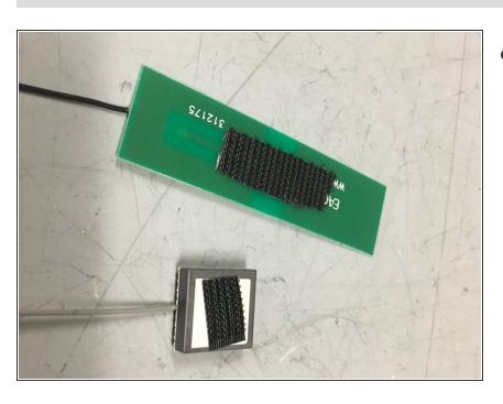
Attach rough-sided velcro on the antenna and GPS as shown in the picture.
