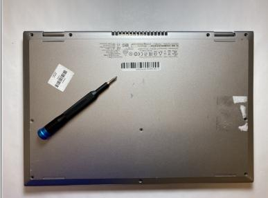
• Use a Phillips #0 screwdriver to remove the ten 8mm screws from the back case of the laptop.
