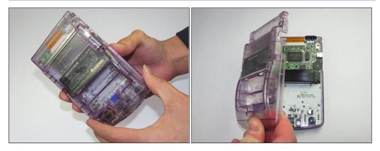
• Gently lift and separate the back housing from the rest of the device. Now you've got the back housing out!
