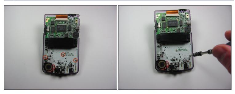
• Using the Phillips #1 screwdriver, remove the 3 screws shown in the picture.
