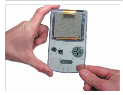
• Remove the original buttons from the housing.
