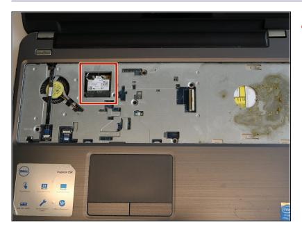
Once the keyboard is removed, the Wi-Fi module will be accessible.
