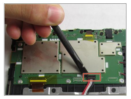
• With slight force pry off the cable connecter using a spudger.
