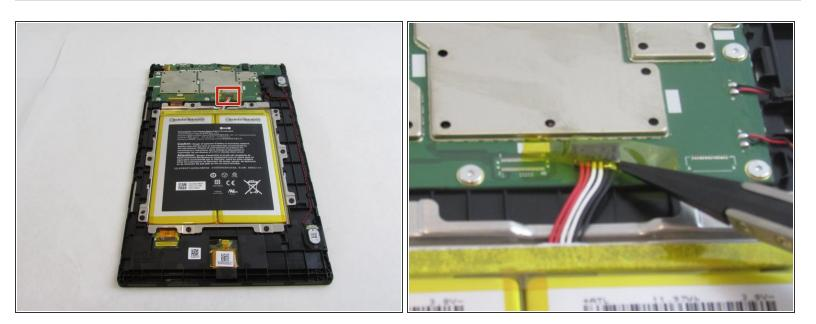
• Remove the plastic yellow taping from the wire circuits using a pair of tweezers.
