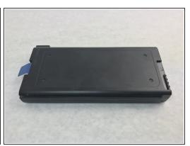
Use the blue tab to pull the battery out of the battery compartment. Make sure to keep the battery latch tab depressed while doing so.
