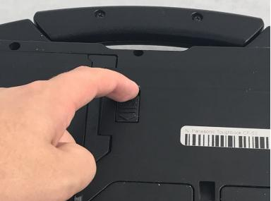
Use the battery release slider to release the battery latch.
