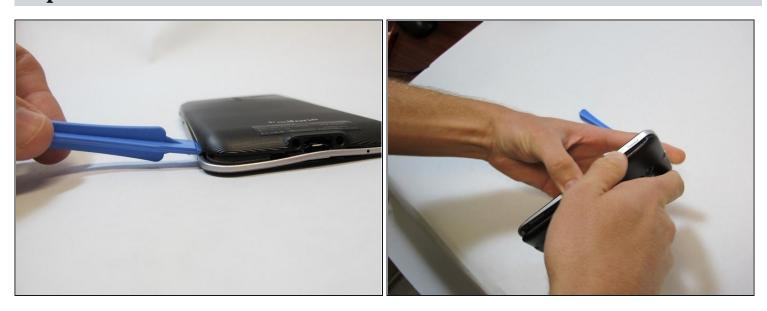
Use plastic opening tool to pry off the back cover of the phone.
