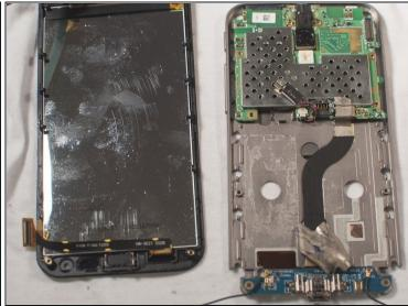
• Place your plastic opening tool at the side of the screen. Make sure all chords are unplugged and not stuck anywhere. Remove the screen from the metal frame.
