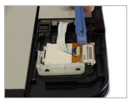
After removing the top cover of the LCD assembly, remove the LCD using the plastic opening tool.
