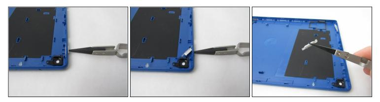
Use tweezers to remove and pick up the button carefully.
