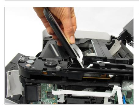
Gently pull the LCD screen up to remove it from its fixture.
