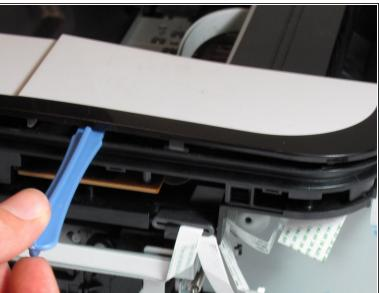
Using the plastic opening tool, gently pry around the cover behind the LCD screen to remove it from its fixture.
