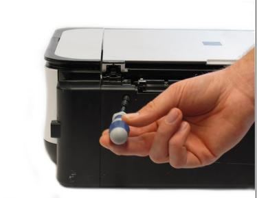
Remove the two 7.9 mm screws using a Phillips #1 screwdriver.
