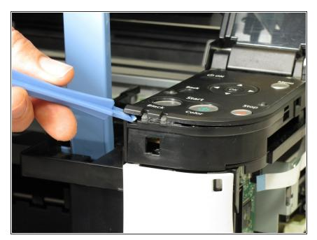
Using the plastic opening tool, gently pry around the button cover to remove it from its fixture.
