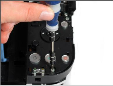
• Remove the five 7.7 mm screws using a Phillips #1 screwdriver.
