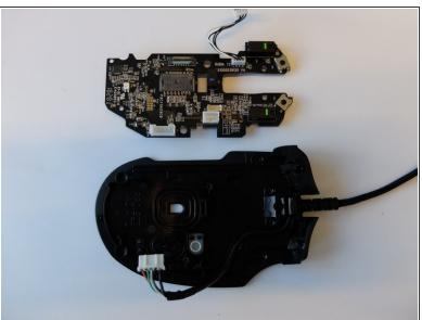
Remove four 3mm JIS #1 screws holding the main board.
