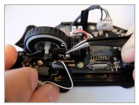
Remove the scroll wheel feedback bar from the scroll wheel by holding down the spring and using angled tweezers to remove it from its placement.
