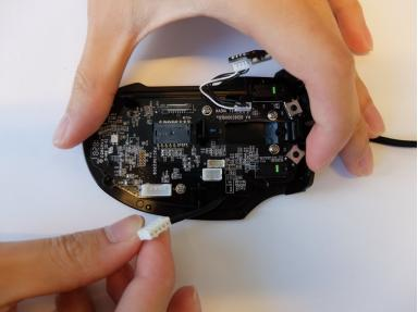
Remove the USB Type A to 5-pin connector from the main board by pinching and pulling upwards.
