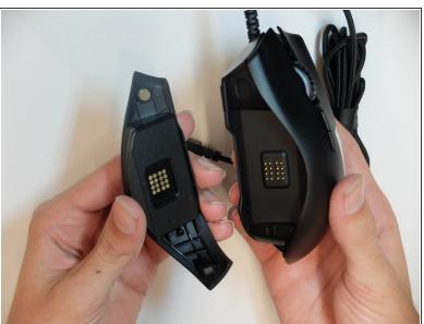
Remove the interchangeable side plate.
