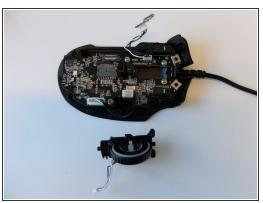
Using the opening tool, pry the black bracket holding the scroll wheel in place backwards until the scroll wheel housing pops out.
