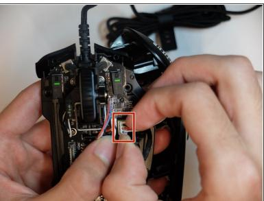
Remove the top housing LED 3-Pin connector that is near the main board.
