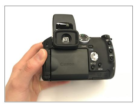
Remove the back cover of the LCD screen (has "Canon" written on it).
