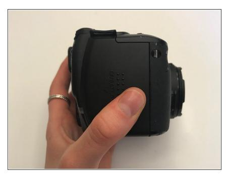
Locate the battery compartment cover on the right hand side of the camera. The cover features the text: "CF/BATT.OPEN".
