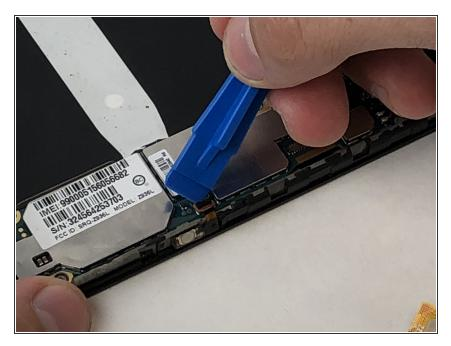
Disconnect the power button from the motherboard with a plastic opening tool.
