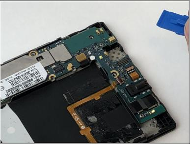
• Use a plastic opening tool to flip up the retaining flap on the volume ribbon cable **ZIF** socket.
