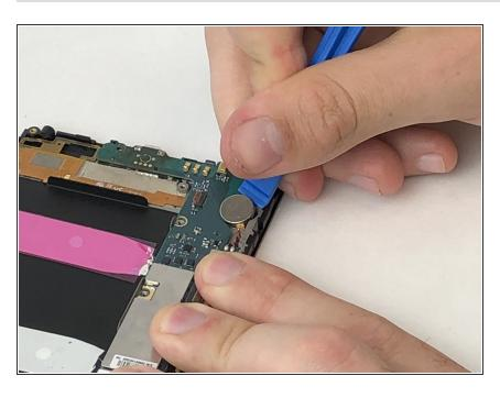
Pry the motherboard cell battery from its position on the case of the phone
