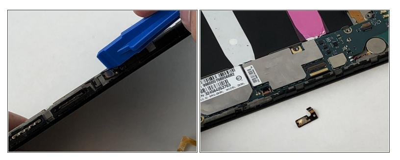
Peel the power button cable up from the phone with you hands, or a plastic opening tool.
