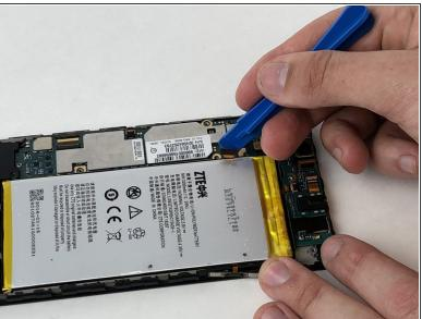
Disconnect the battery cable from the motherboard with a plastic opening tool.
