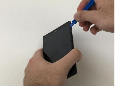
Use an iFixit opening tool to separate the back from the device.
