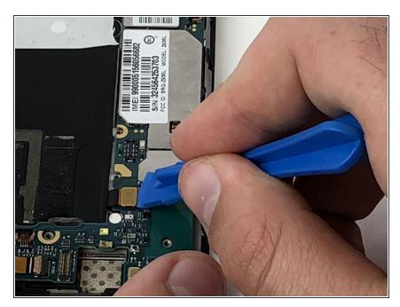
Disconnect the display cable from the motherboard with a plastic opening tool.
