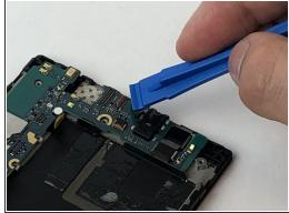
• Disconnect the camera from the motherboard with a plastic opening tool.
