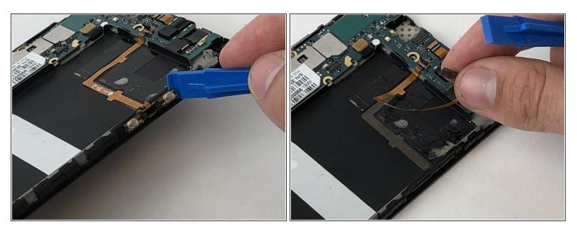
Peel up the volume button cable from the phone with hands, or plastic opening tool.
