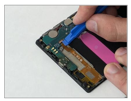
Disconnect the rear speaker cable from the motherboard with a plastic opening tool.
