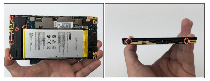
Remove the seven 1.6mm Phillips #0 screws from the plastic cover on the bottom of the motherboard.
