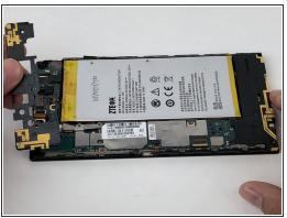
Remove the top plastic motherboard cover using a plastic opening tool.
