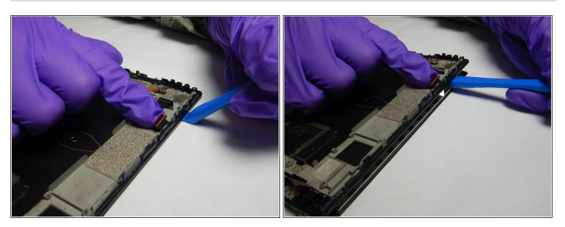
Using the iFixit opening tool, pry off the screen from the case.
