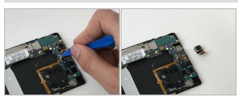
Disconnect the camera from the motherboard with a plastic opening tool.
