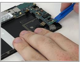
Using the plastic opening tool, pry the motherboard up, sliding along the edge to separate the pieces.
