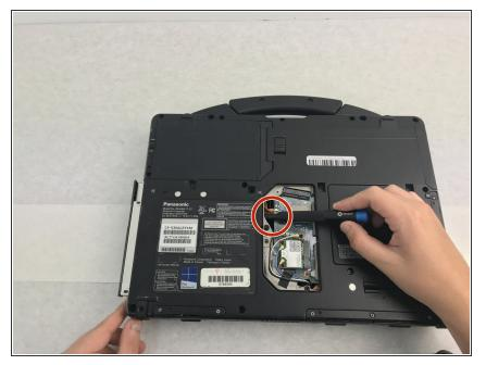
Reach under the silver tab and push the optical drive out of the side of the device using a spudger.
