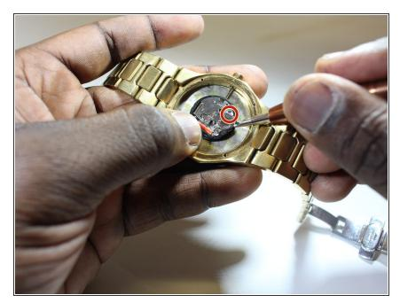
Loosen the battery bracket from the watch by placing the 1mm flathead screwdriver under and lifting carefully.
