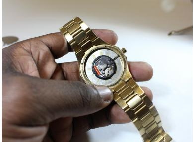
Take the old battery out using the plastic opening tool or spudger.
