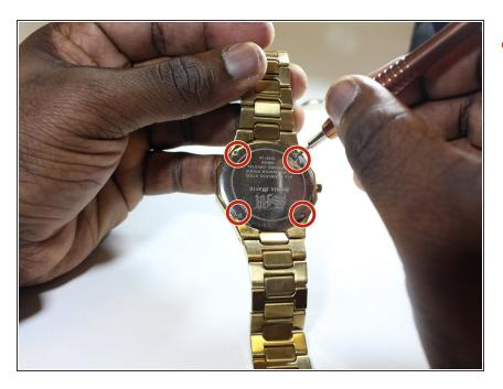
Remove four screws from the back cover using the Y000 screwdriver .
