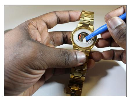
Remove the plastic gasket from on top of the battery using the opening tool.
