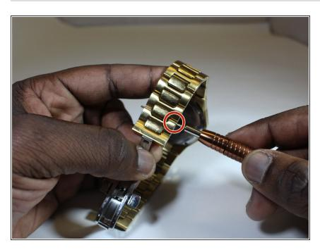
Take apart the steel strap for the watch by using the round head (SIM) screwdriver. Then pull out the screw.
