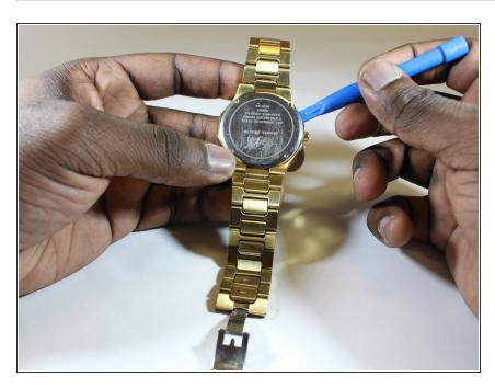
Remove the back cover of the watch using the opening tool.
