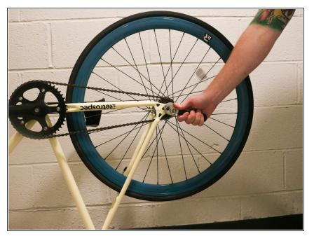
Remove the 9.5mm bolts on the rear wheel with an adjustable wrench. There is a bolt on each side of the wheel.
