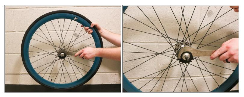
Remove the lockring on the back tire using a lockring wrench. To loosen the lockring twist the wrench clockwise.
