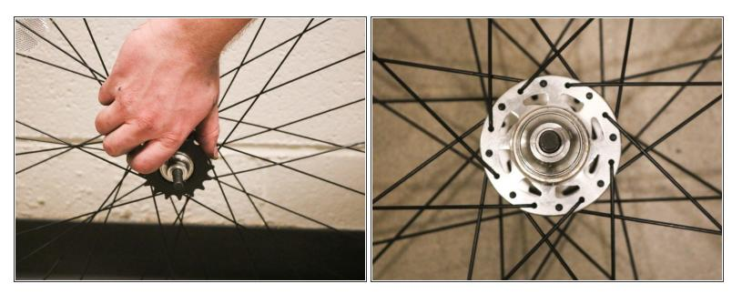
Remove the cog the rest of the way with your hand. Replace with a new cog.
