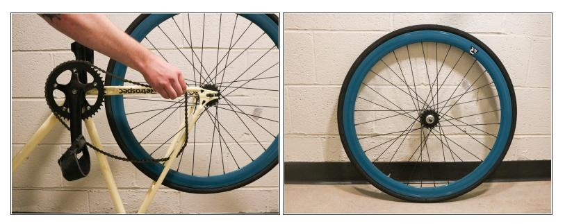
• Remove the chain from the rear wheel cog. Remove the rear wheel from the frame of the bike.
