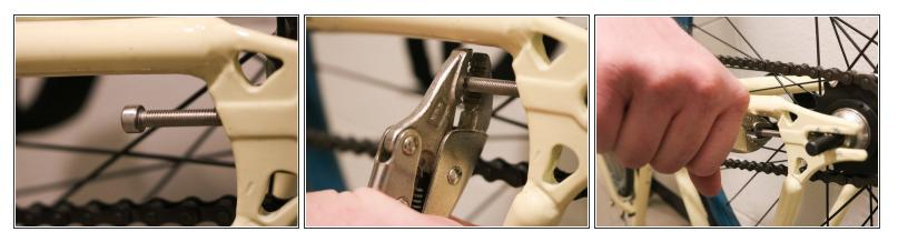
Loosen the 4mm by 50.8mm chain tension screw with a hex key. There is a screw on each side of the wheel.
