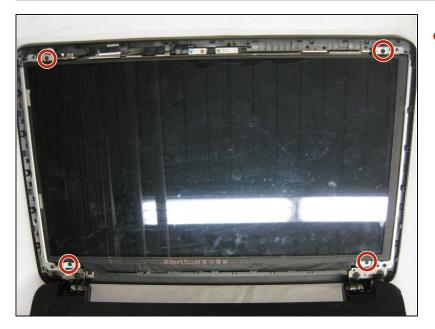
Using a Phillips #000 screwdriver, remove all four 2mm screws in each corner of the screen.
