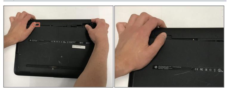
• To remove the battery, slide the left slider on the back to the unlocked position.
