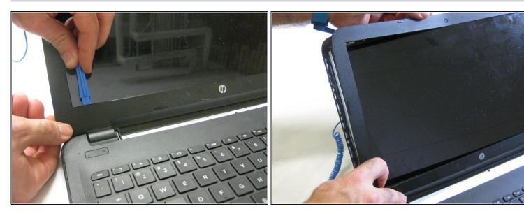
• With the screen facing you, use the plastic opening tool to remove the liner around the screen
