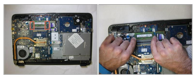
Using your fingers, carefully release the locking devices on both sides of the RAM card by moving them away from each other.
