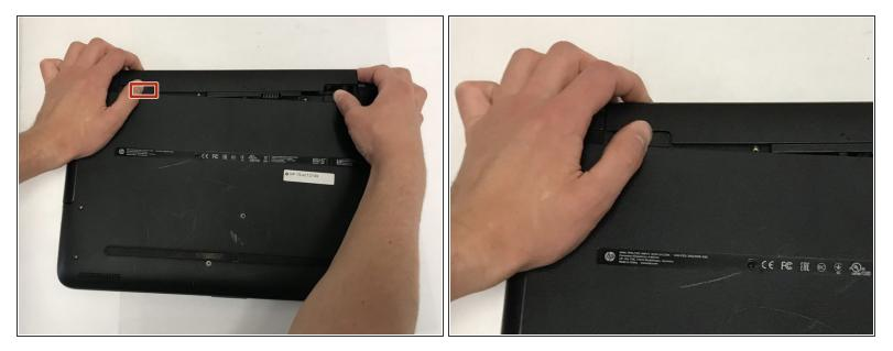
• To remove the battery, slide the left slider on the back to the unlocked position.
