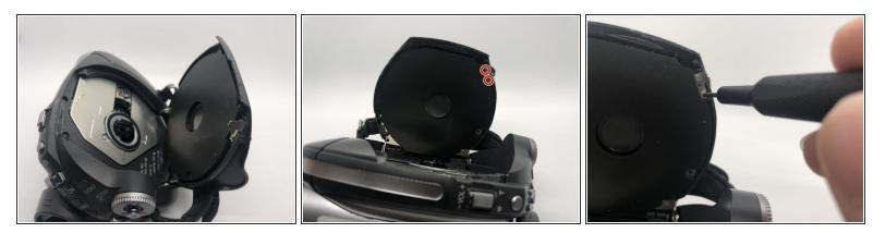
• Remove the two 5mm screws on the top-right corner of the disk slot using Phillips #0 screwdriver.
