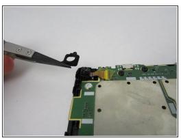
Remove the rubber casing around the camera lens using a set of tweezers.
