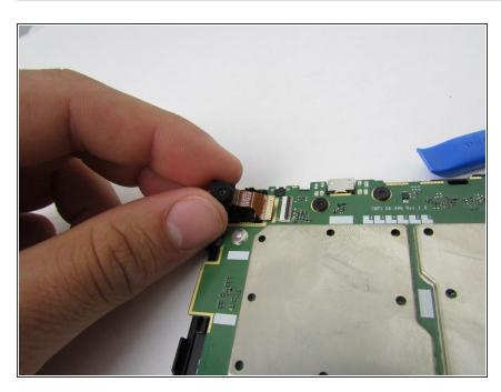
Remove and pull off the camera lens.
