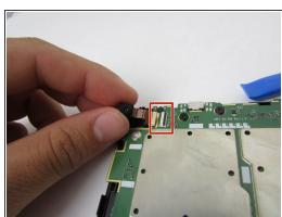
Gently flip over the black latch with the iFixit opening tool. Disconnect the camera's connector to the circuit board.
