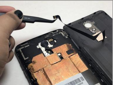
Use the tweezers to pull at the base of the film to remove the fingerprint scanner.
