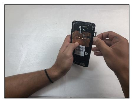
Remove the SD and SIM cards by pulling out the card tray from the slot on the right side of the device.
