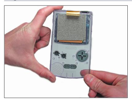
Remove the original buttons from the housing.
