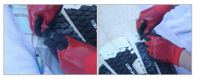
Using a razor blade, cut away at the adhesive under the traction pad.
