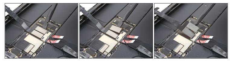
• Use a spudger to pry up and disconnect the two bottom display cable press connectors.
