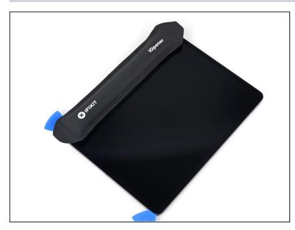
• Apply a heated iOpener to the left edge of the screen for two minutes.
