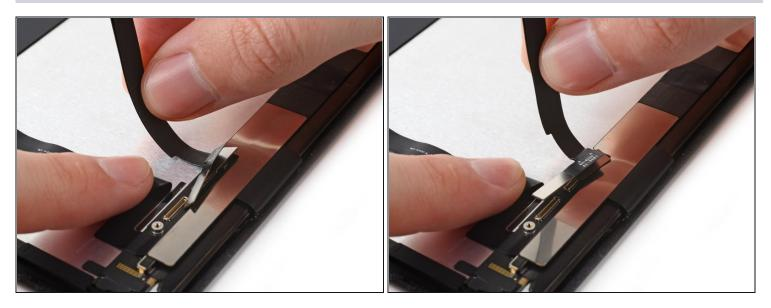
(i) The display cable is lightly adhered to the screen.
