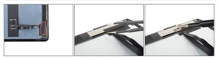
• Peel back the tape from the display cable bracket located at the bottom right of the screen.
