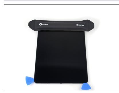
• Apply a heated iOpener to the top edge of the screen for two minutes.
