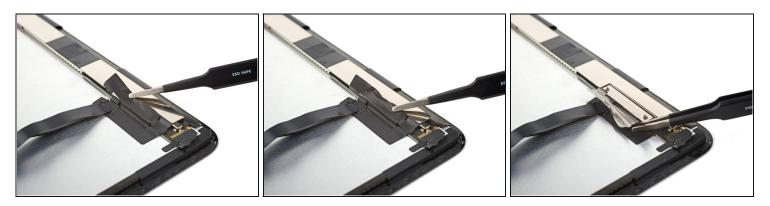
• Continue peeling the tape along its outer edge until the bracket is fully exposed.
