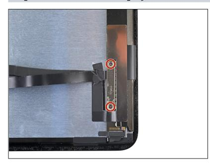
• Use a Phillips screwdriver to remove the two 1.3 mm-long screws securing the display cable bracket.
