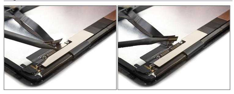
• Use a spudger to pry up and disconnect the top display cable press connector on the screen.
