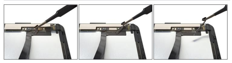
• Peel off the tape connecting the display and digitizer cables.
