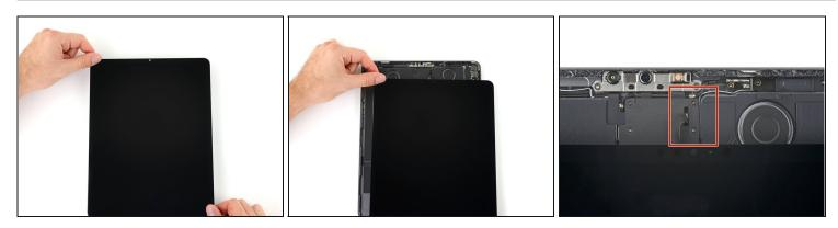
A Don't fully remove the screen, as it's attached to the frame by several cables.
