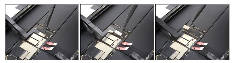
• Use a spudger to pry up and disconnect the two top display cable press connectors.
