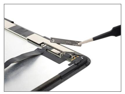
• Remove the display cable bracket.
