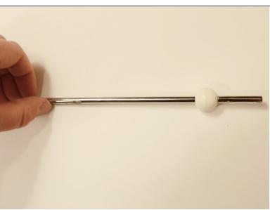
Pull the pivot rod out to expose the ball. Remove the whole pivot rod fixture.
