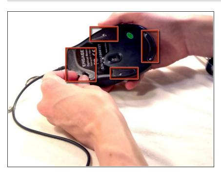
Flip the mouse over and peel off the stickers on the perimeter of the bottom of the mouse.
