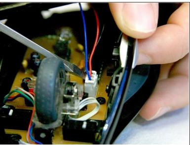
Use a spudger to pry underneath the white plug and pop it out to disconnect the upper board from the lower board.
