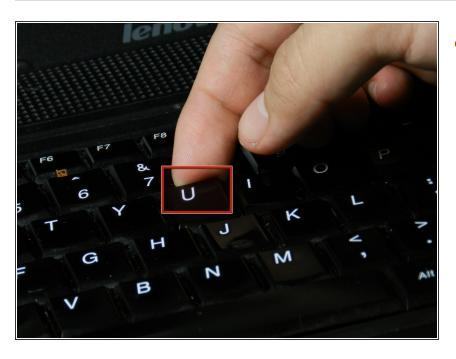
Place your pointer finger under the key you want to remove. For extra leverage, use the thumb and rotate the key in the manner shown.
