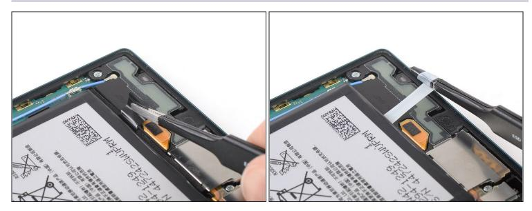
• Use a pair of tweezers to pull out the second adhesive strip from underneath the battery.
