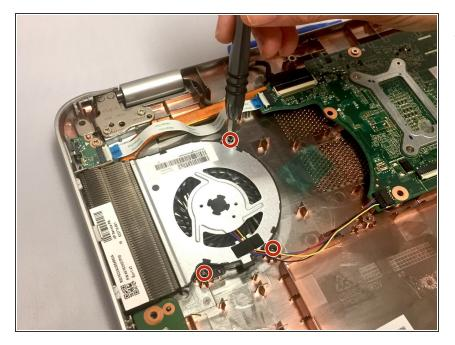
Remove the three 4mm screws using the Phillips #0 screwdriver from the device fan.
