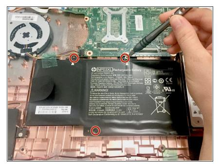
• Remove the three 4mm screws using the Phillips #0 screwdriver.
