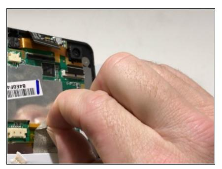
Peel back the metallic tape connecting the motherboard to the tablet body with your fingers.
