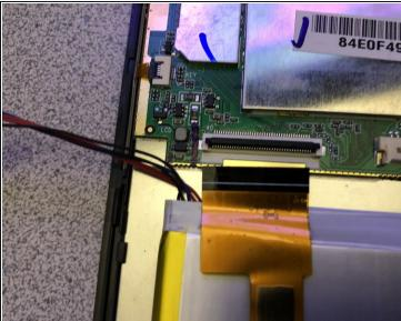
Opening the locking tab of the ZIF connector and carefully remove the upper section of the ribbon cable from the motherboard using tweezers.
