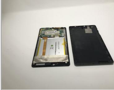
Remove the backing of the tablet to reveal the internal components using a plastic opening tool.
