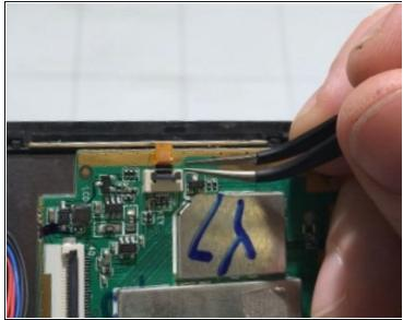
• Disconnect the three remaining ribbons by opening the locking tabs of the ZIF connectors and gently pulling the cables out.
