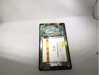
Remove the silver/metallic tape covering the blue and red wires overlapping the upper and lower end of the ribbon cable.
