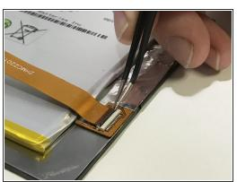
Remove the ribbon cable by pulling the locking tab of the ZIF connector up and pulling the ribbon cable out with tweezers.
