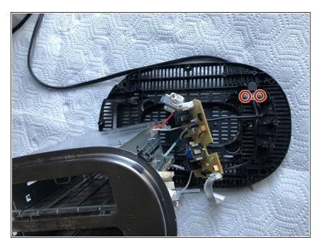
Pull apart toaster components. If power cable needs to be removed or adjusted, unscrew the screws circled.
