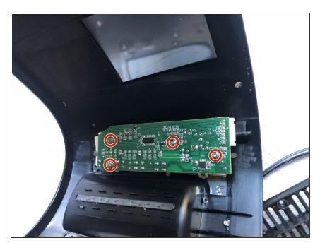
If the circuit for the buttons and shade selector needs to be removed, unscrew these 4 screws.
