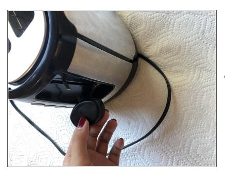
Remove bread lifter/toast booster by prying it off. The plastic piece snaps over the metal part during assembly. Use a flat-blade screw driver from the side to widen the gap in the plastic clip while pulling the plastic handle out. Done right the handle can later be reassembled securely.
