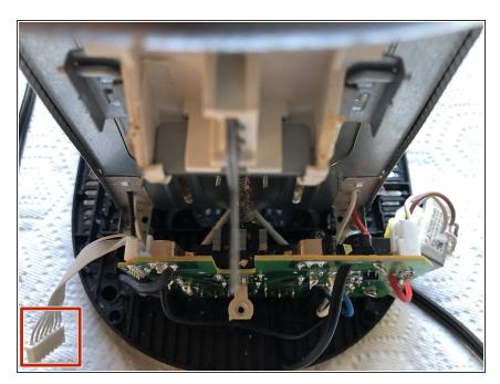
Disconnect the two circuits by unplugging the wires shown. This can be done by pressing the lever on the crimps. Then the shell can be pulled off from the rest of the toaster.
