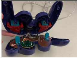
Carefully pry open the controller. Ensure that the rumble assembly stays intact.
