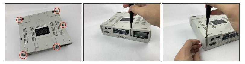
Remove the five black 13.5mm JIS#1 screws on the bottom of the device. One might be hidden by a sticker.
