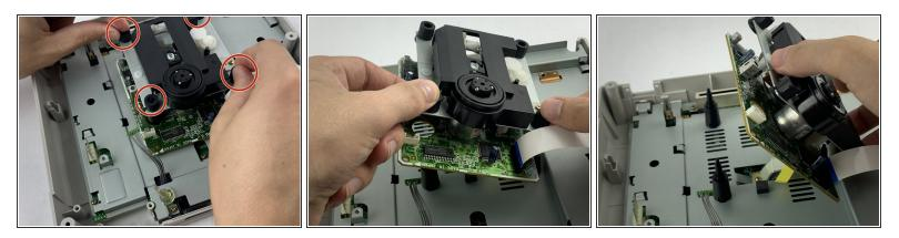
• Lift the laser reader slowly out of its slot hosted by these four pins. There is a screw underneath with a cable attached to the motherboard.
