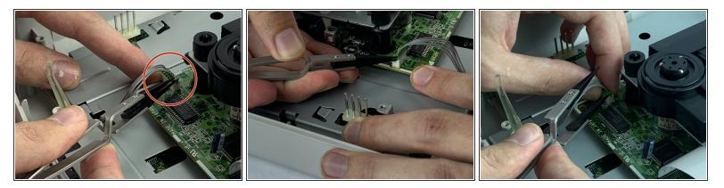
Pry the second cable out of its socket on the disk reader with the iFixit opening tool or ESD safe tweezers. When the lip of the cable gets enough distance out of the socket, it can be wiggled free.
