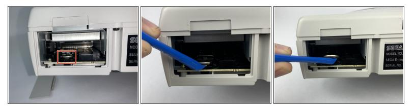
• Push up the edge of the battery with the iFixit opening tool to get the battery out of its socket.
