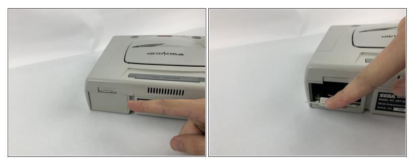
• Press on the plastic lever on the back of the Sega Saturn to pop open the battery slot.
