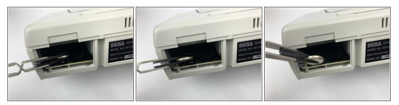
• Use the ESD safe tweezers to pull the battery out of its slot.
