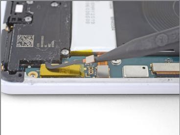
• Use the point of a spudger to pry up and disconnect the loudspeaker connector from its motherboard socket, near the bottom right edge of the phone.
