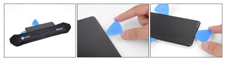
Continue heating and slicing until you have sliced around the entire perimeter of the phone.
