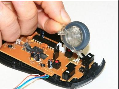
Pop the scroll wheel out of the snap holding it in place. You can use your finger or a spudger to do so.
