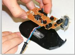
Lift the bottom board up to remove from its mounting posts. This will separate it completely from the bottom panel of the mouse.
