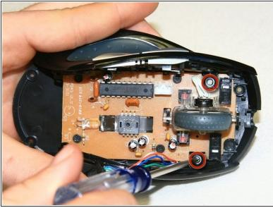
Locate the 5 mm silver flat head mounting screws (2) to the left and right of the scroll wheel and remove with the Phillips #1 screwdriver.
